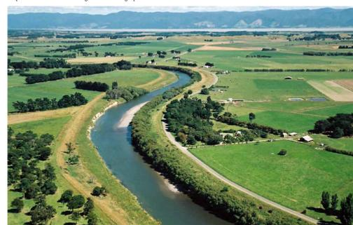
The stopbanks have been built to different standards primarily because of funding shortages.
